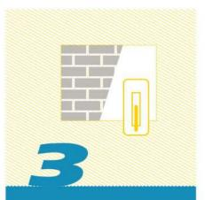
Plaster according to Lightweight Block plastering procedures with a thickness about 5-10 mm.
